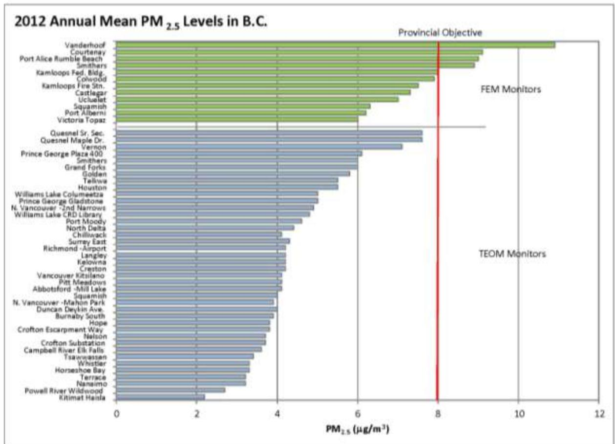
Figure 5: Summary of PM<sub>2.5</sub> levels in BC in 2012. Data from two sets of monitors are shown: from the older TEOM instruments (blue bars) and the new FEM instruments (green bars) (2013 State of the Air, BC Lung).
